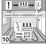
**Preparation:** Please store the packets 48 hours prior to installation under the same climatic conditions (temperature and moisture) as the actual installation process [1]. Important pre-condition for proper fitting and long-term durability of the laminated flooring is a room temperature of 15 - 30°C / 59 - 86°F and a relative humidity of around 40 - 70%.
