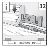
In order to avoid splintering of the edges, the decorated side should face down when using electrical jigsaws or hand-held circular saws. Otherwise, cut down from the top of the panel. Begin each new row with the remnants (at least 30 cm / 12" in length) of the previous row.
