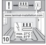
**Preparation:** Please store the packets 48 hours prior to installation under the same climatic conditions (temperature and moisture) as the actual installation process [1]. Important pre-condition for proper fitting and long-term durability of the laminated flooring is a room temperature of  $15 - 30^{\circ}\text{C} / 59 - 86^{\circ}\text{F}$  and a relative humidity of around 40 - 70%.
